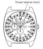
The power reserve indicator shows the amount the watch is wound as an amount of time, so you can see how long the watch will run at a glance. The power reserve hand indicates the remaining amount. The time pointed to by the power reserve hand is the remaining amount of time.
