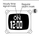
With each press, the engagement and disengagement of the regular alarm and hourly time signal are made as follows:
